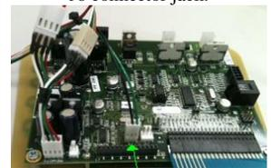
Green and white wire couple plugged into J6 connector jack, with additional Y-Pig-Tail housing both red and white Wi-Fi or Blue Tooth receiver and 20 function remote receiver.
