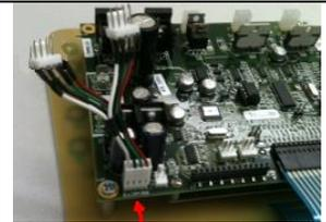
Y-Pig-Tail attached to 4-prong Remote connector jack.
