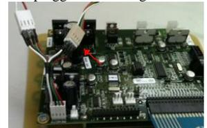
20 function remote receiver plugged into Y-Pig-Tail
