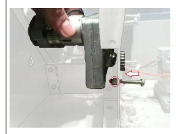
**Step 5.)** Hold the new motor into position with one hand, (Make sure the motor is Top is at its highest elevated point), and proceed to fasten the 4 screws down.
